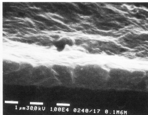
Figure 12. Scanning electron micrograph of a cross section of a polyaniline film prepared from a 0.1 \mu\text{m} outside diameter PANi tubules.
